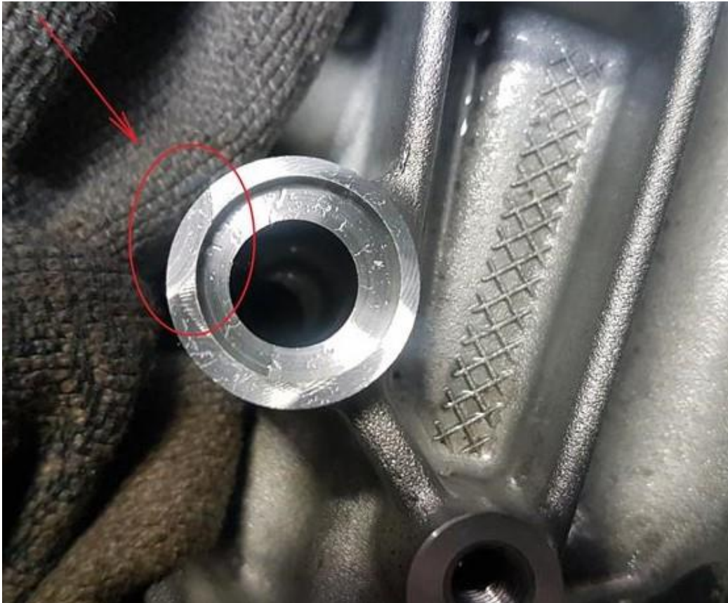
Figure 1. OGC oil cooler connection beveling grooves.
