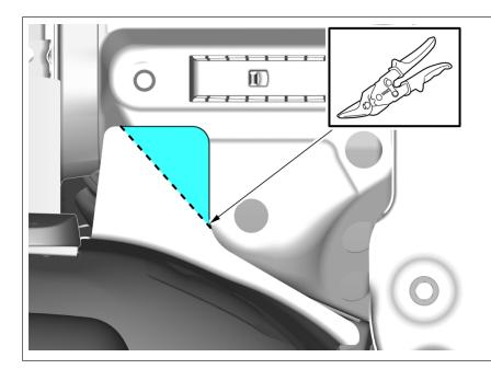
**Use:** Sheet metal shears Remove the marked part. On both sides.
