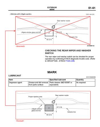
Please make the indicated changes to the 2018 Mirage Service Manual, Group 51-Exterior -> Windshield Wiper and Washer -> Removal and Installation.
