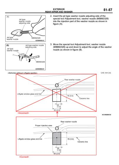
Please make the indicated changes to the 2014 Mirage Service Manual, Group 51-Exterior -> Windshield Wiper and Washer -> Removal and Installation.
