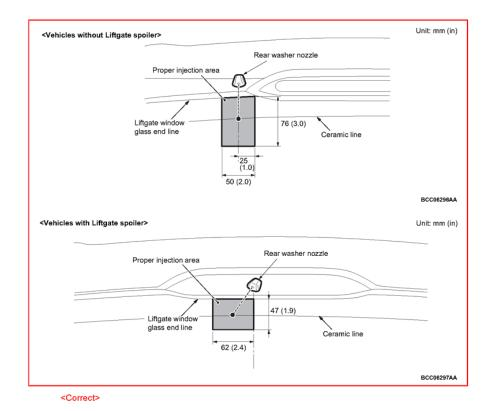
Please make the indicated changes to the 2019 Mirage Service Manual, Group 51-Exterior -> Windshield Wiper and Washer -> Removal and Installation.
