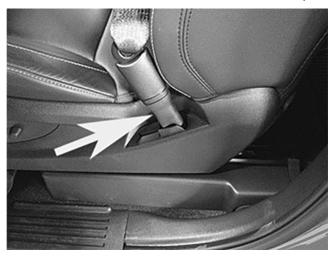
2. Inspect the seat belt tensioner cable cover for damage. Inspect the complete cable cover from the base of the cable to the buckle.
