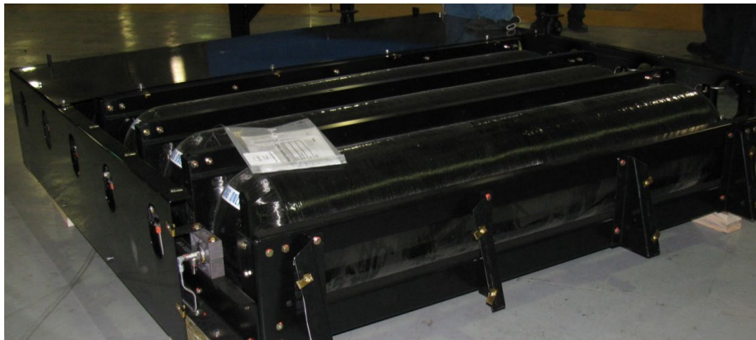
Figure 5. Type 4 CNG cylinders in a housing with the cover partially removed. PRDs are located at each valve and at various locations along the length of the cylinder.
