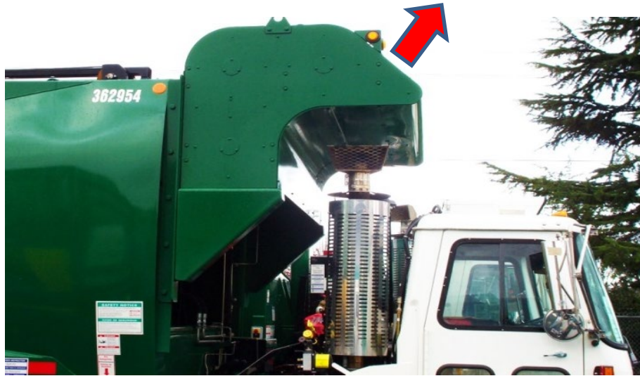
Figure 8. CNG PRD venting location and direction (arrow), front of body refuse system.
