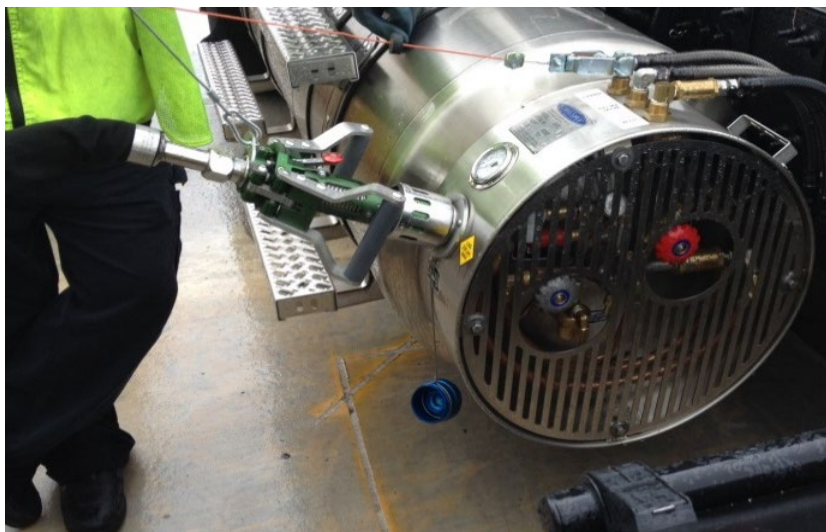
Figure 13: LNG fuel tank valve end with protective shield installed. NOTE: Driver side shown; passenger side similar.
