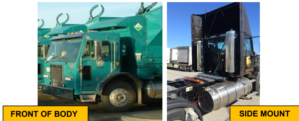
Figure 3c. Two LNG fuel system configurations offered by Agility ® .
