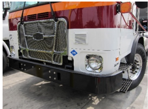
Figure 1a. Left: CNG fueled vehicles are identified by a blue and white decal on the right rear of the vehicle. Right: A CNG decal may also be affixed to the left front of the vehicle.
