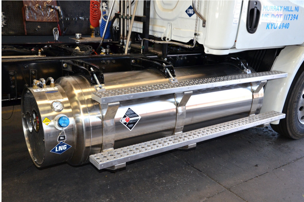
Figure 12. Stainless steel LNG fuel tank with LNG blue diamond decal. NOTE: Passenger side shown; driver side similar.
