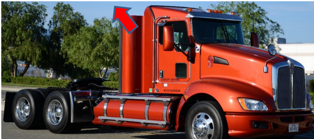
Figure 6a. CNG PRD venting location and direction (arrows), side mount and behind the cab systems.
