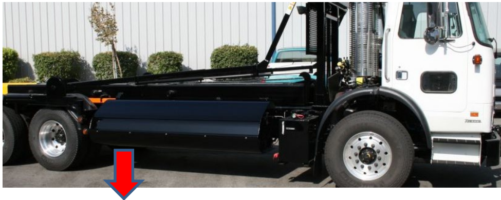
Figure 6c. CNG PRD venting location and direction (arrow), older side mount systems.
