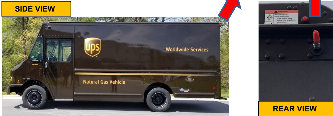
Figure 6b. CNG PRD vent tube outlet location and vent directions (arrows), medium duty side mount system.
