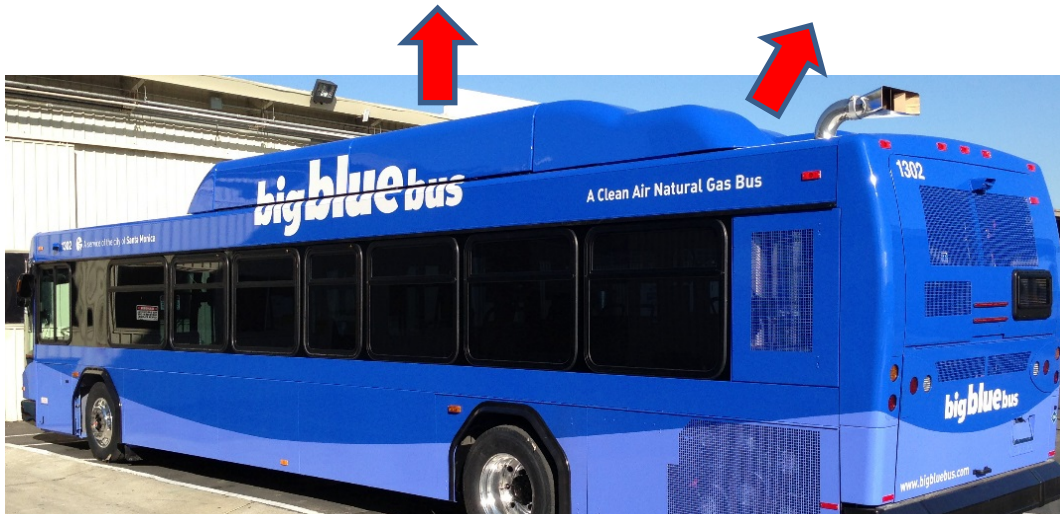
Figure 9. CNG PRD venting locations and directions (arrow), transit bus.
