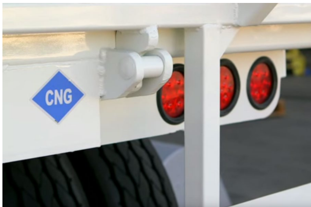
Figure 1a. Left: CNG fueled vehicles are identified by a blue and white decal on the right rear of the vehicle. Right: A CNG decal may also be affixed to the left front of the vehicle.
