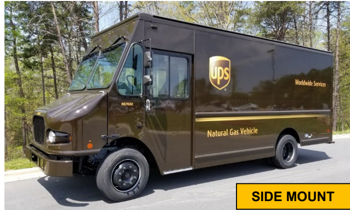
Figure 3b. Medium duty Agility ® CNG side mount fuel system. NOTE: CNG fuel cylinders (not visible) bolt to chassis frame rails and are protected by vehicle body and shields.
