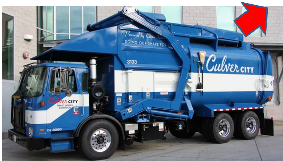
Figure 7. CNG PRD venting location and direction (arrow), refuse roof mount systems.
