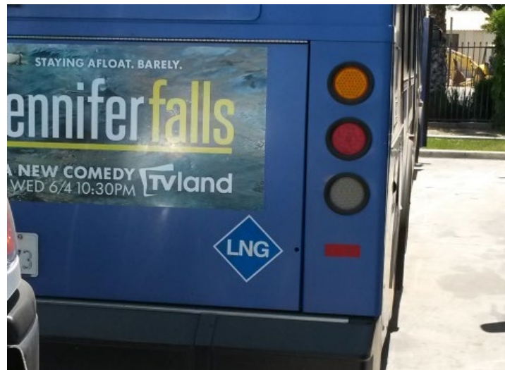
Figure 1b. Top: LNG fueled vehicles are identified by a blue and white diamond decal. Left: LNG blue diamond decal location on lower right rear of cab on vehicles without bodies such as roll-off refuse haulers. Right: LNG decal on the side mount fuel tank. Bottom: LNG decal on the right rear of a transit bus.
