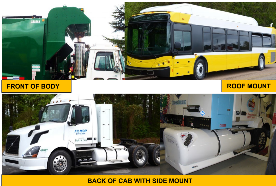
Figure 3a. Popular heavy duty Agility ® CNG fuel system configurations.
