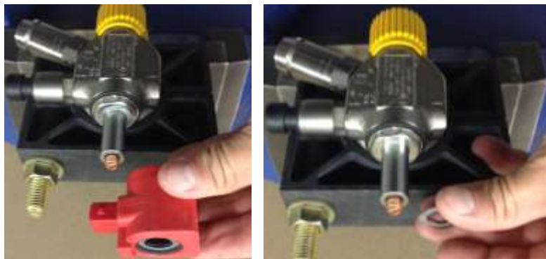
Figure 6. Left: Coil slides off valve stem. Right: Remove spring washer.
