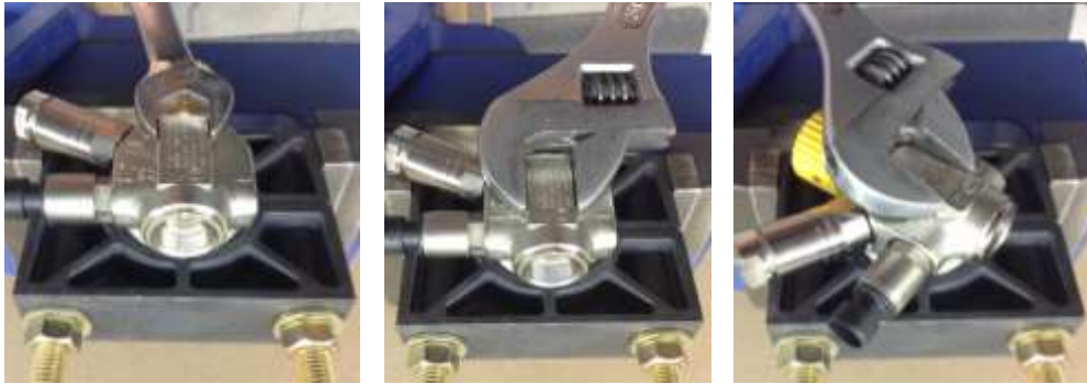
Figure 11. An adjustable wrench may be used to remove valve from cylinder.
