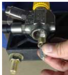
Figure 8. Remove spring and plunger.
