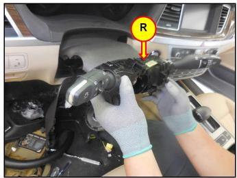
19. Remove the multifunction switch assembly (R).
