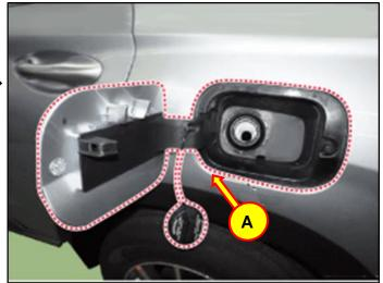
2. Remove the existing fuel filler door panel (B) from the fuel filler door housing (C).
