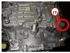
Remove the plug (1) from the old transmission to be re-installed in the new transmission.
