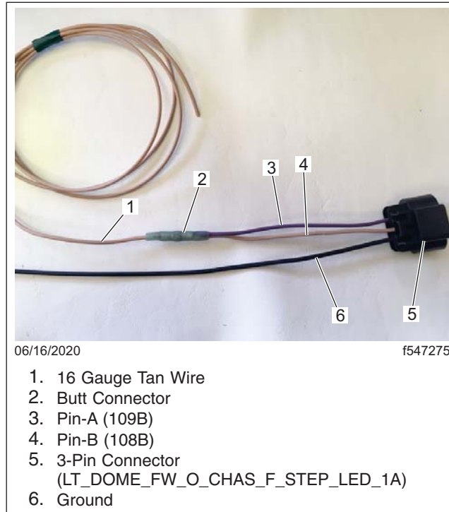
Fig. 3, 3-Pin Connector after Splicing
