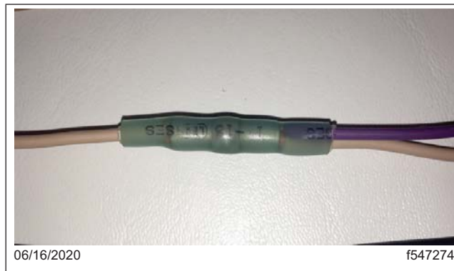
Fig. 6, Butt Connector Heat Shrunk
