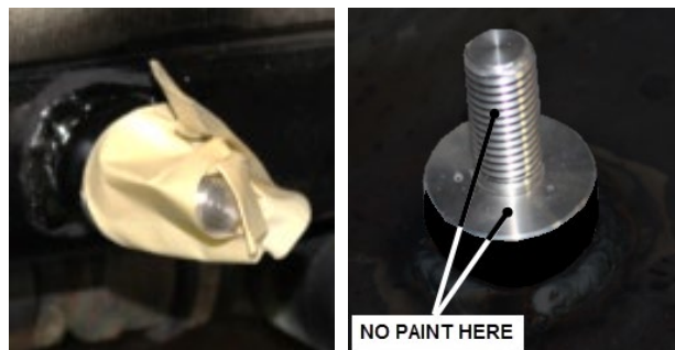
FIGURE 79: GROUND STUD #380360
