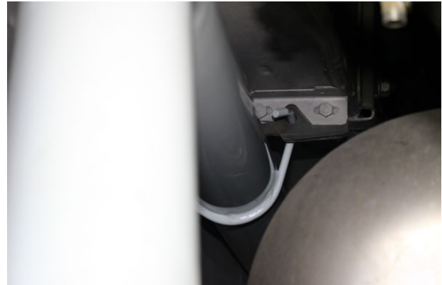
FIGURE 99: ENGINE INTAKE PIPE SUPPORT
