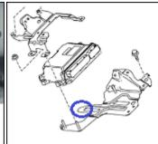
To eliminate this concern, the shape of the PCM bracket has been modified to not cover the breather hole and eliminate a gap between it and the PCM that may promote the residual liquid wax.
