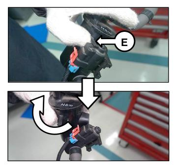
6b. Remove the canister close valve from the fuel tank air filter by turning the valve clockwise.
