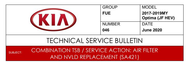
This bulletin provides the procedure to perform an evaporative leak test and replace the fuel tank air filter, and, if necessary, the Natural Vacuum Leak Detector (NVLD) on some Optima (JF HEV) vehicles, produced from June 27, 2016 through January 7, 2019, which may experience an evaporative leak concern with DTC P0456. Before conducting the procedure, verify that the vehicle is included in the list of affected VINs.
