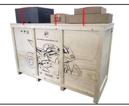
2. To open the crate, it is necessary to remove the **48 self-tapping screws** that fix the 4 walls and the cover together. <u>We suggest proceeding by starting from the cover and then</u> <u>moving on to the side walls.</u>
