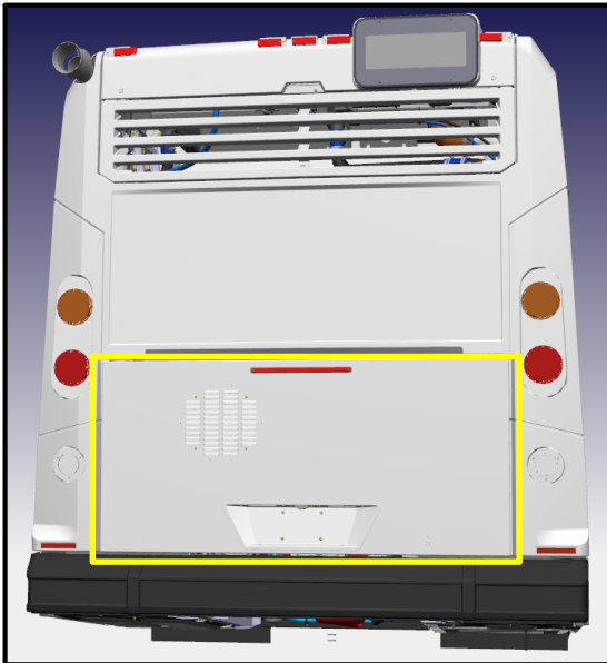
Figure 2 – Rear Door Compartment
