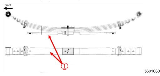
Note: The part number is stenciled in yellow and stamped in the metal on the bottom of the helper spring.
