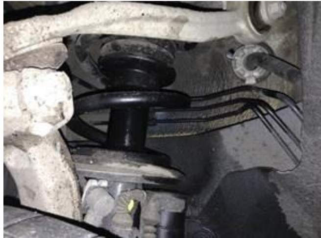
Figure 2, 3, and 4. Oil marks/residues in the wheel housing/shock absorber.
