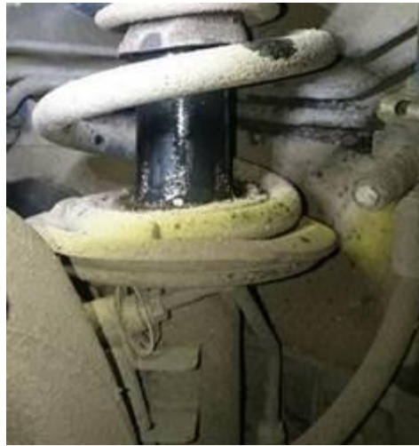
Figure 1. DRC shock absorber with clear oil loss.
