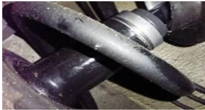
Figure 1. DRC shock absorber with clear oil loss.
