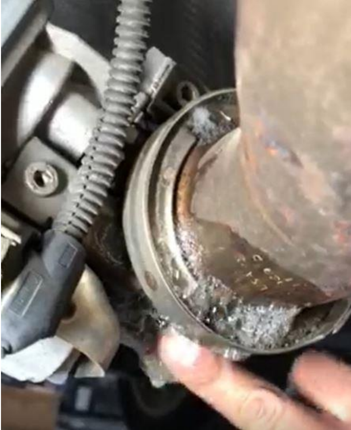
Figure 1. Example of exhaust leak at exhaust flap.
