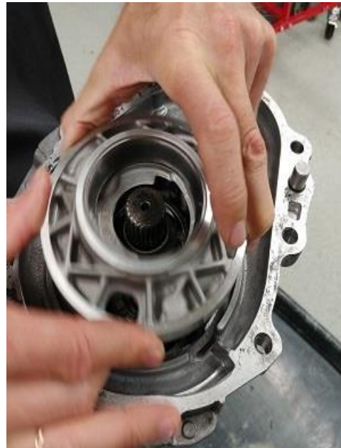
Figure 10. Gear carrier removal.
