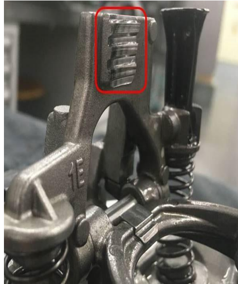
Figure 1. Worn/faulty shift fork.
