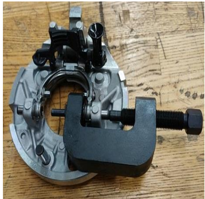
Figure 18. Pin pressing with the 582277.
