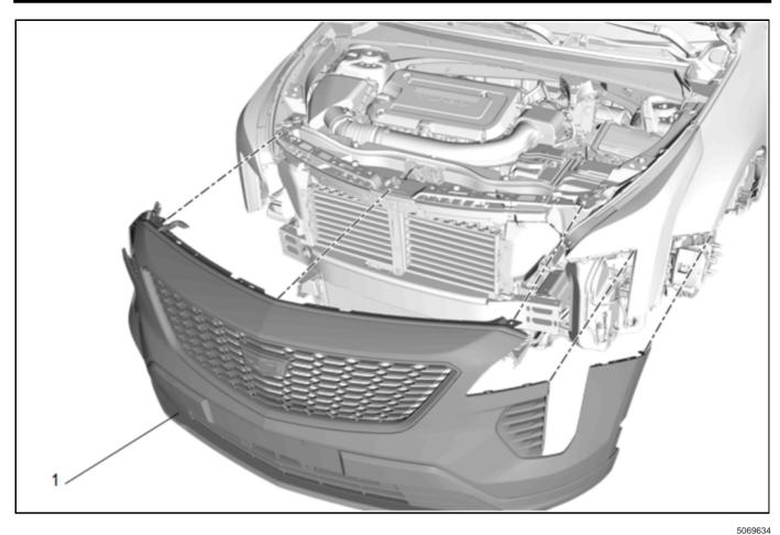
6. Reinstall the front fascia (1). Refer to *Front Bumper Fascia Removal and Installation* in SI.
