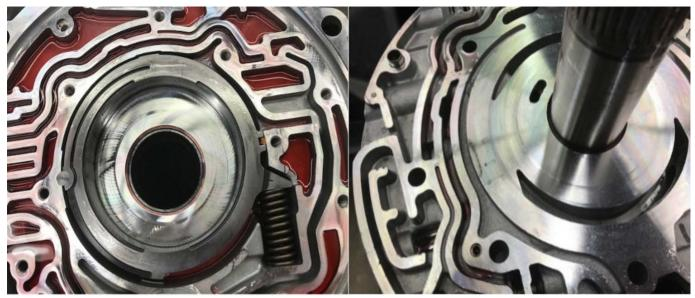
**Do Not** replace the pump if no signs of damage or excessive wear was not validated during inspection as shown above.
