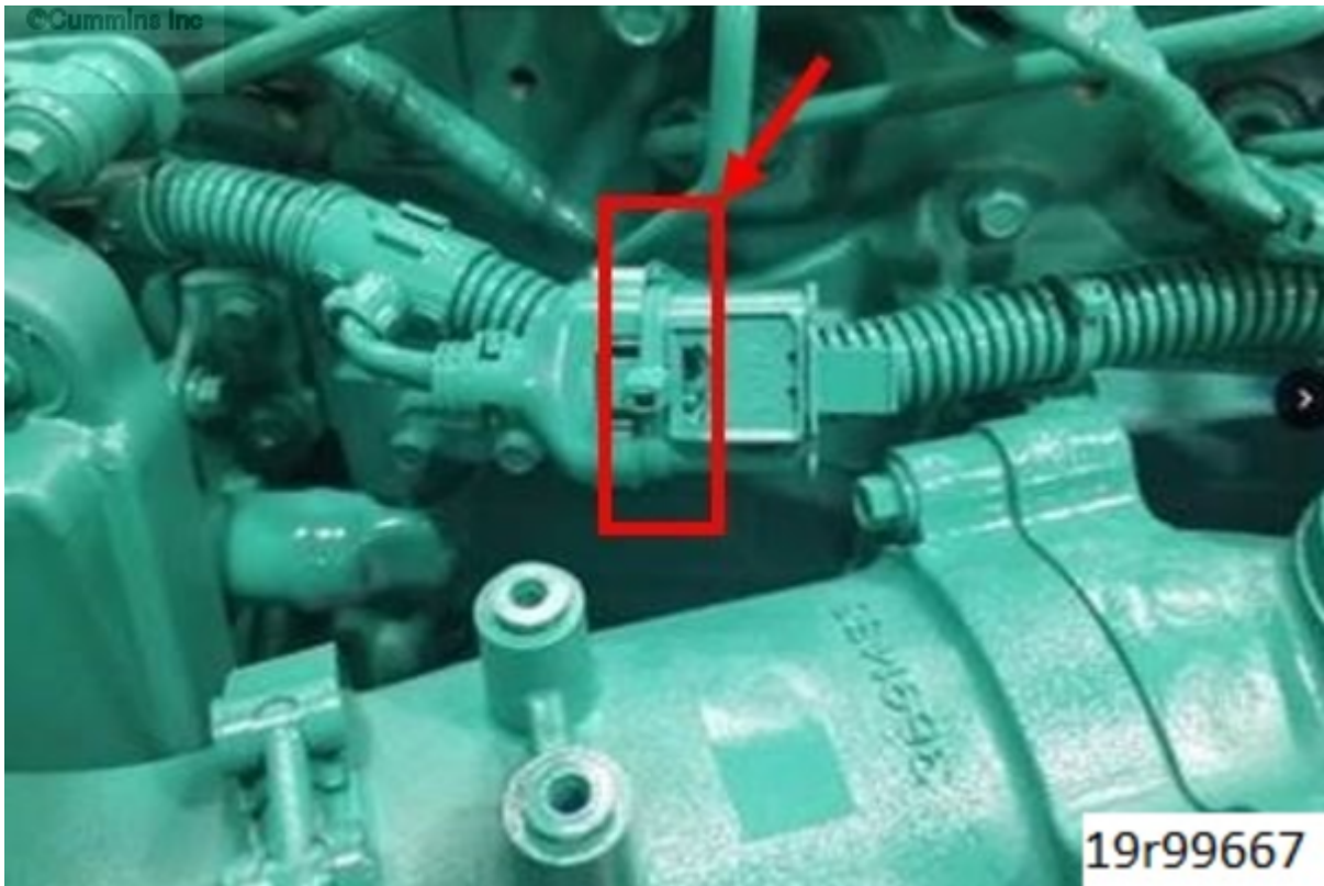
Figure 4, Correct Orientation of Connector
