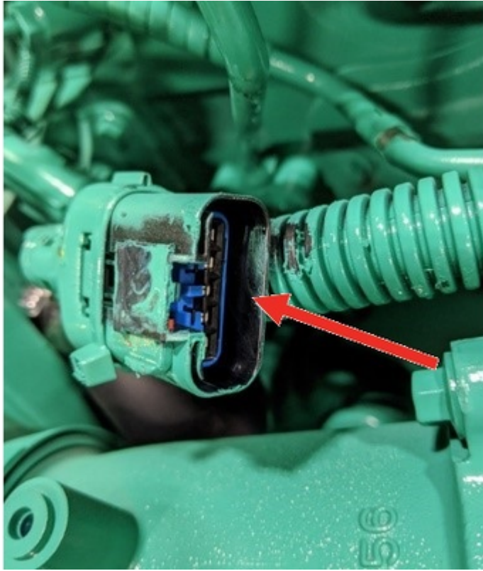
Figure 2, Blow Out Excess Water
