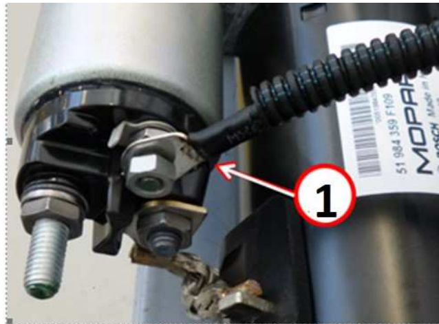
Fig. 9 Starter Wiring Installed
