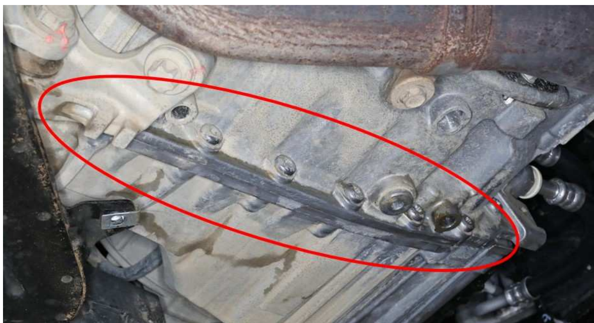
Fig. 2 (Reference Picture) Potential Leak Area at Case Split
