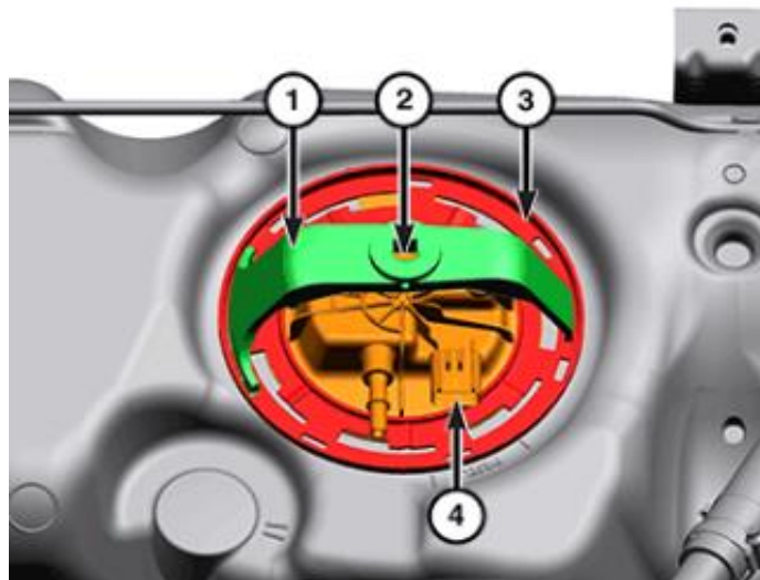
Figure 5 – Fuel Pump Lock Ring Wrench 9340
