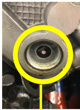
Overheated Pink Sensor 255°F Coolant Temp
