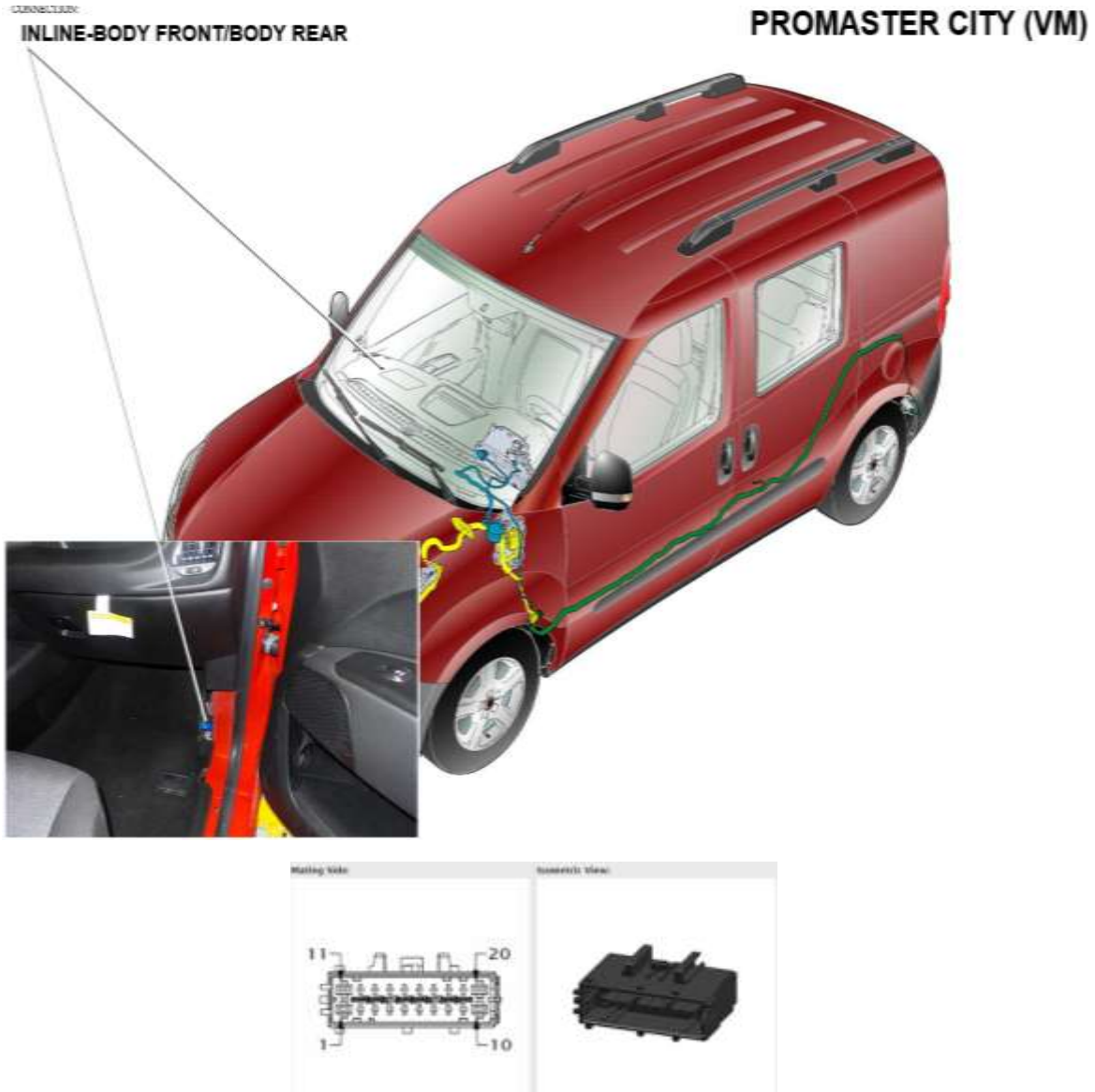
Fig 4, I008B connector location/20-way black
