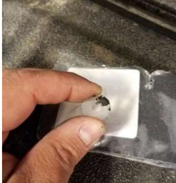
Butyl or RTV on washer to hold it in place for assembly
