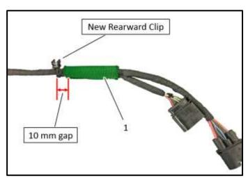
Install the new protective sleeve <1> around the wiring harness.
