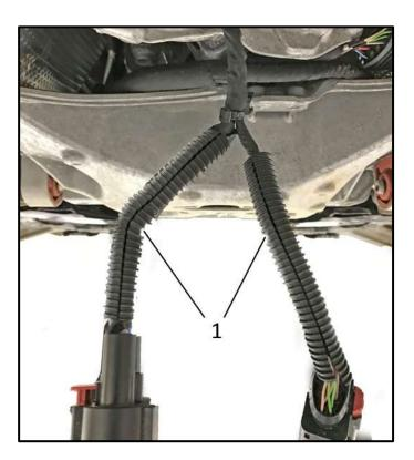
Install 130 mm of corrugated tube <1> onto each <u>body side</u> wiring harness section as shown.
