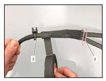
Wrap the protective sleeve with fabric tape.
