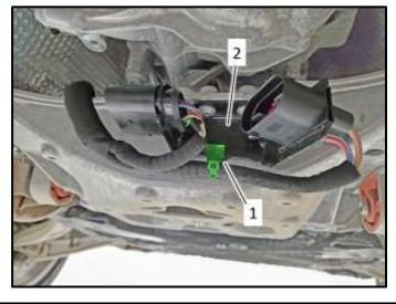
Install new wiring harness clip <1> onto harness as shown and secure to connector bracket.
