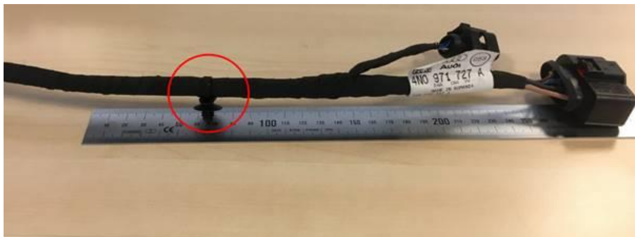
Figure 3. Clip to be removed from the old or new harness.
