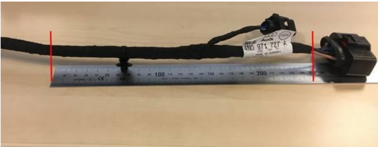
Figure 4. Add additional wrapping between the two red lines, approximately 250mm.
