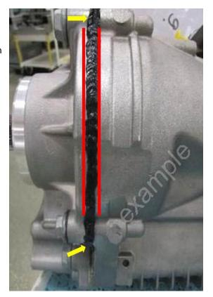
Figure 4. Silicone sealant application.
