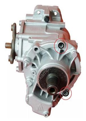
Figure 5. Silicone sealant at bolt holes.
