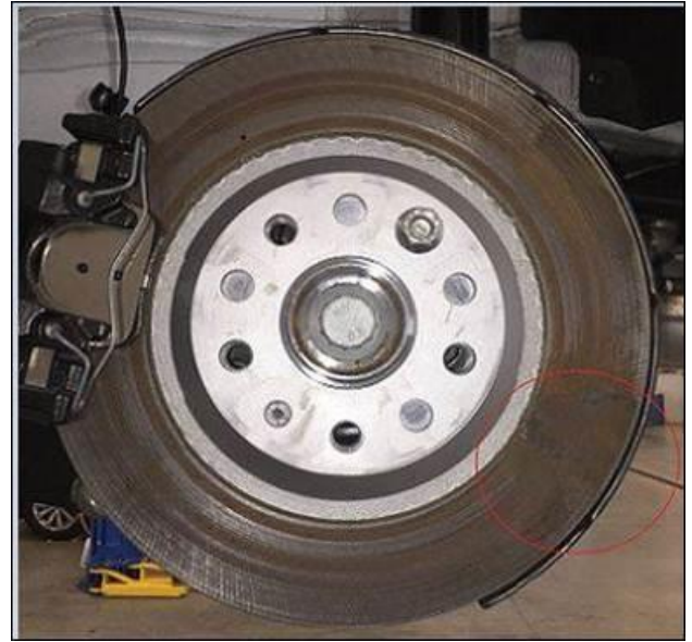
Figure 8: Corrosion, brake pad stuck to brake disc.
