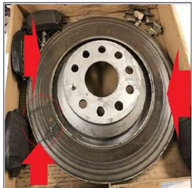
Figure 6: Corrosion, brake pad stuck to brake disc.
