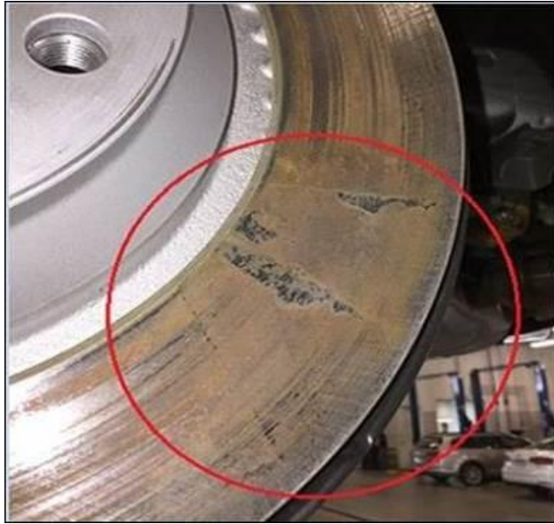
Figure 7: Corrosion, brake pad stuck to brake disc.
