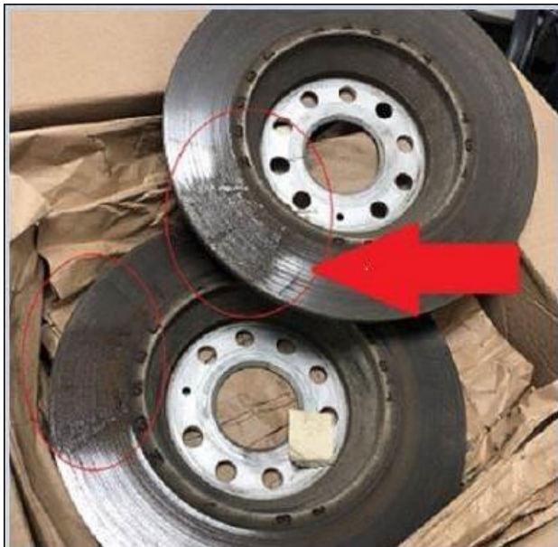
Figure 9: Brake Pad stuck to Brake Disc
