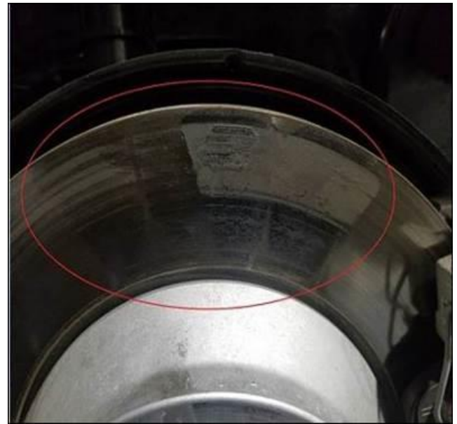
Figure 10: Brake Pad stuck to Brake Disc.
