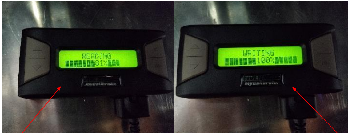
Figure 8: MyCalibrator reading DTCs (14), MyCalibrator writing data to PCM (15).
