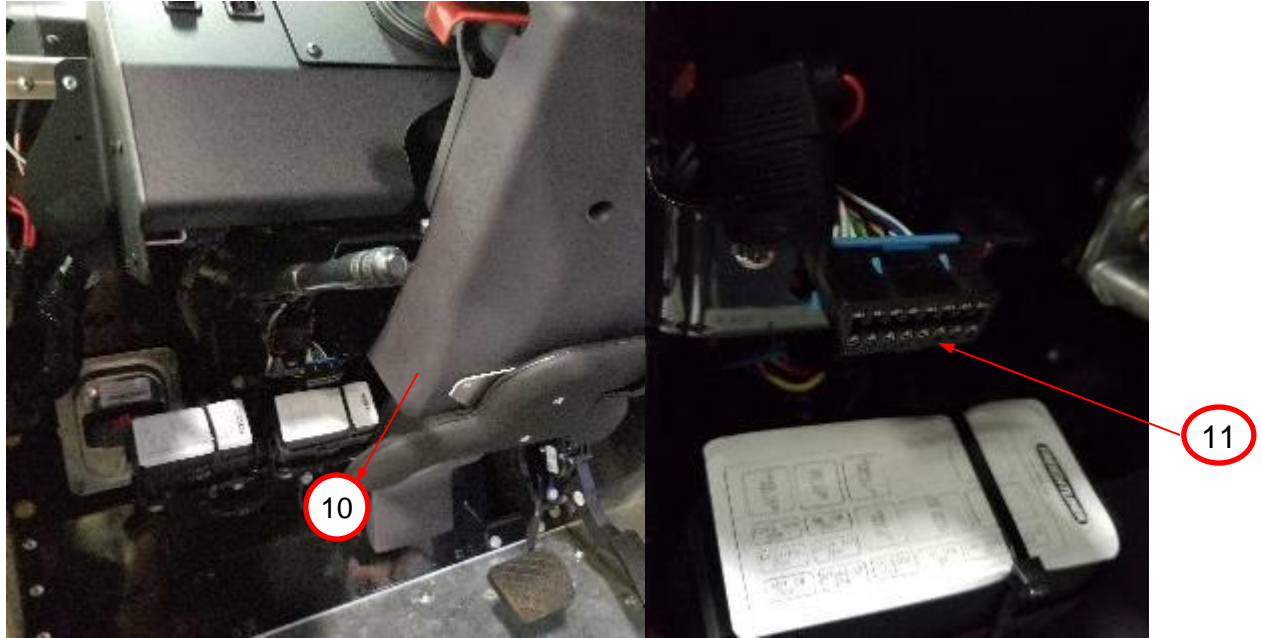
Figure 6: Steering column (10), Data Link Connector (DLC) (11).
