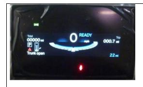
The customer states that the trunk open warning is displayed, even though the trunk is mechanically closed.
