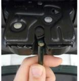
Check the movement of the tailgate lock in both detent positions with a pencil or similar object.
