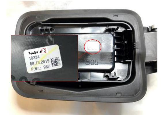
3.Use the P/N and index to determine if replacement is required:
