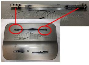
7. Apply a 5 mm section of butyl inside each locking tab of the filler door, in the area shown to the left.
