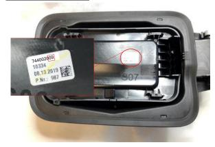
1. Open the fuel filler door to inspect the orientation of the fuel filler door ejector.
