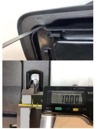
4. Close the filler flap and measure the distance between the upper tab and the filler door assembly. The gap must be at least 0.1 mm.
