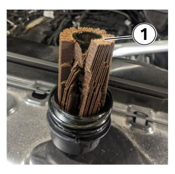
The engine oil filter is broken. The paper is torn, and the lower plastic section is stuck in the engine oil filter housing (1).
