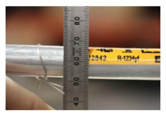
If the TXV tubes on the new evaporator are bent down order a new evaporator and return the damaged part as "new defective". Do not attempt to adjust the tubes to allow installation of the evaporator in the HVAC case. If the tubes are bent or adjusted back into position this will result in a slow leak from the lock ring joint.
