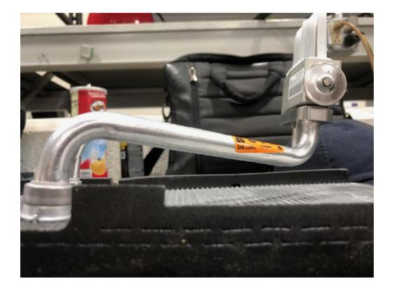
There should be a distance of 60 mm. when measuring from the core to the center of the TXV tubes as shown below.
