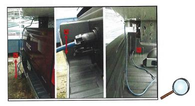
3. Poor trailer wiring connections, as shown below. General Motors does not recommend these type of connections, but many trailers utilize these connections. These type of connections are not robust and are not recommended, especially for brake wiring.
