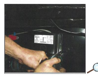
5. The CCM/BSCM is detecting the wrong type of trailer brakes. This is normally caused by an aftermarket device wired into the trailer. The example shown below is an electric over hydraulic-to-electric brake adapter. These adapters are used to make a truck that only works with electric trailer brakes work with a trailer that has electric over hydraulic brakes.
