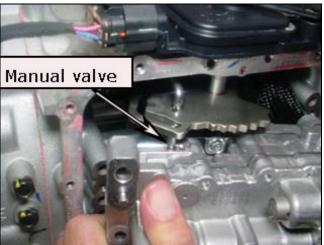
20. Install the valve body bolts and torque the bolts to specification in the order shown.
