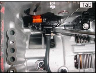
17. Remove two bolts that secure the valve body harness to the case.
