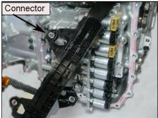
13. Pull the solenoid connector outward and move the connector out of position.
