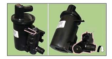
13. Install the new air filter KIT and reinstall the removed parts, including CCV, in reverse order of removal.
