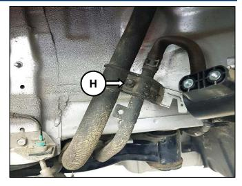
7. Release the hose clamp and disconnect the ventilation hose (I) from the Nature Vacuum Leak Detection (NVLD) valve.
