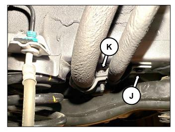
9. Remove the filler neck vent line, upper hose and air filter.
