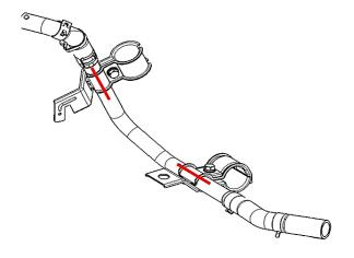
14. Spray the black undercoating aerosol evenly to each vent line bracket for approximately 10 seconds.
