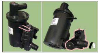
13. Install the new air filter KIT and reinstall the removed parts, including CCV, in reverse order of removal.
