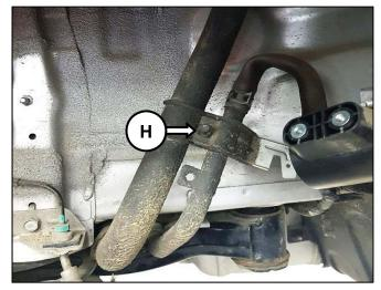
7. Release the hose clamp and disconnect the ventilation hose (I) from the Nature Vacuum Leak Detection (NVLD) valve.
