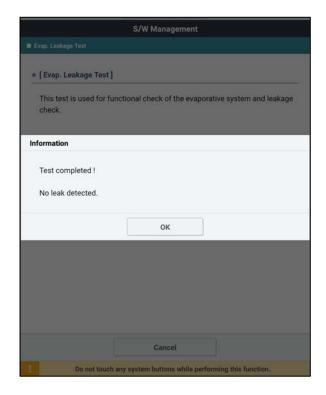
17. Check for installed parts and hose connections if EVAP leakage is detected.
