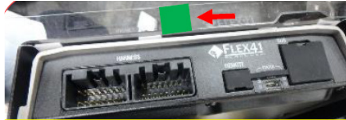
Example of the cap cover from the jumper harness visual configuration. In this example "green" was used for Legacy Premium Models.
