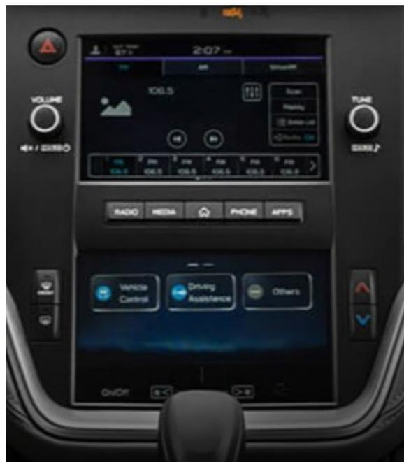
**NOTE:** High Level unit is equipped with Navigation option (Map icon on Home screen)
