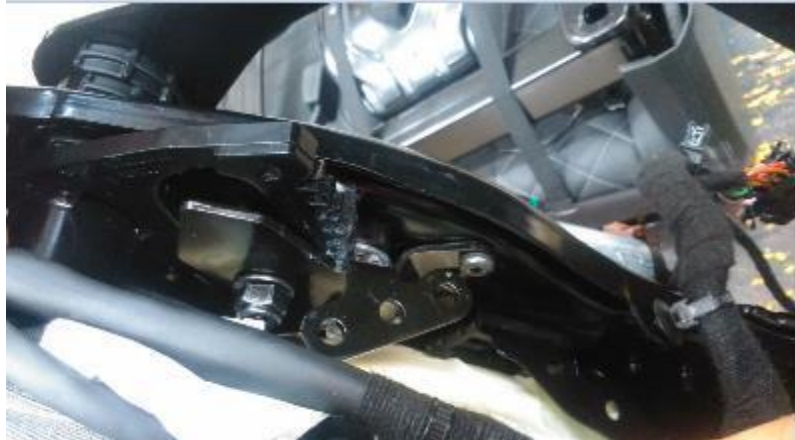
Figure 2. Toothed segment of seat height adjustment.
