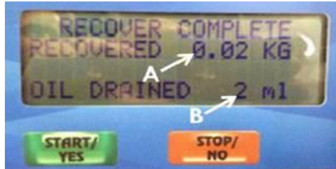
Figure 3: Amount of refrigerant recovered (A), and amount of oil drained (B).
