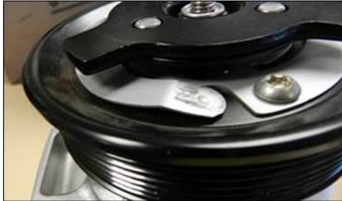
Figure 7a. Example of torque limiter over load protection activated.
