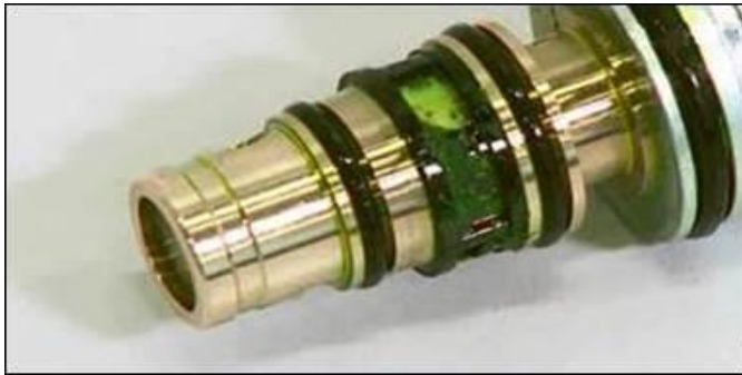
Figure 15: Severe contamination at the -N280- A/C Compressor Regulator Valve filter screen.
