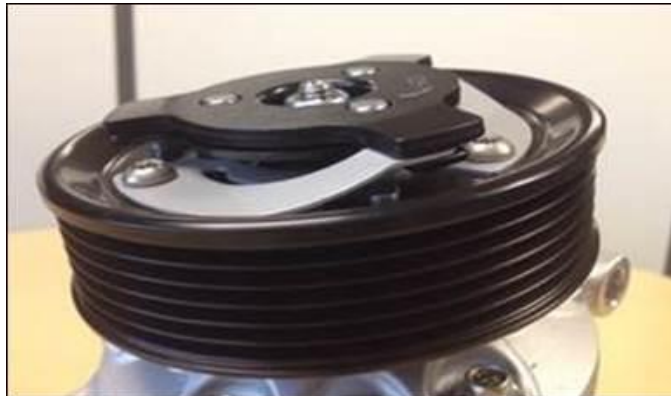
Figure 7b. Example of torque limiter over load protection still intact.
