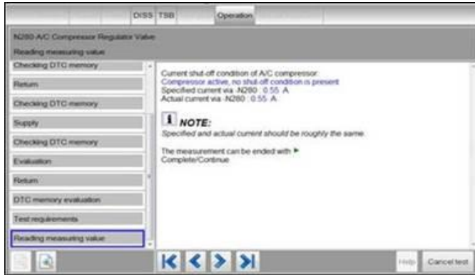
Figure 5. Checking N280 signal value Measuring Value Block.
