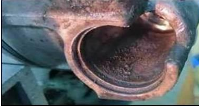
Figure 14. Corrosion in the -N280- A/C Compressor Regulator Valve bore.
