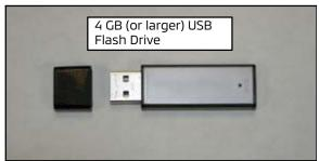
A USB version 2.0 standard flash drive (thumb drive) with a **minimum capacity of 4.0 GB**, formatted to FAT32 is required for this procedure. Formatting to FAT32 will erase all data from the flash drive. The flash drive must have no other files or folders saved to it.
