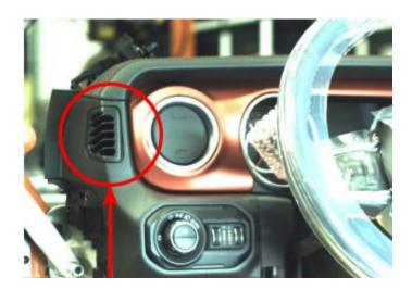
Inspect the demister grill for proper position/installation. Remove the demister grill (side vent cap/cover) inspect the HVAC ducting for proper connections and ensure that it is fully seated and in place. After HVAC duct has been verified to be properly seated and in position, reinsert demister grill. If the demister grill shows visual damage and does not seat properly replace with new.
